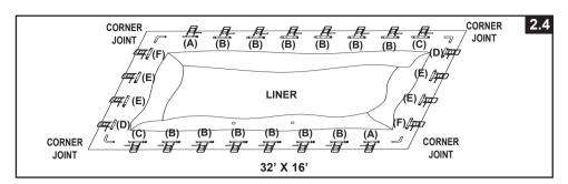
3. Be sure the liner is opened and spread out to its fullest extent on top of the ground cloth. Starting with one side, slide the "A" beams first into the sleeve openings located in each corner. Continue with "B" beam snapping into the "A" beam, and another "C" beam snapping into the "B" beam (see drawing 3).
