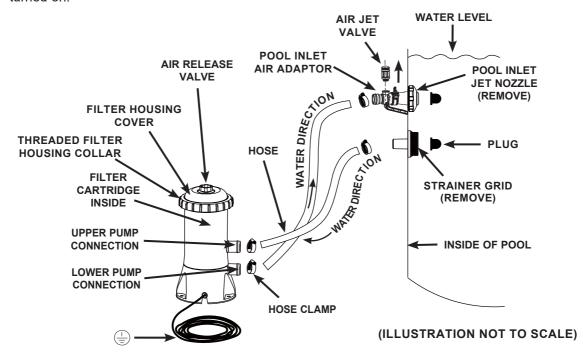
The power cord plug to the 220-240 volt electrical power source of the filter pump must be positioned more than 3.5 m away from the pool walls. Check your local authorities to determine the appropriate standard and requirements for "electrical installation of swimming pools and basins equipment". The following table is for reference only:
